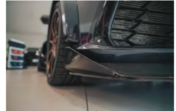
Front Splitter with Winglets
