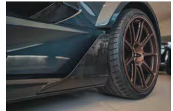
Rocker Extension Guide Vanes
